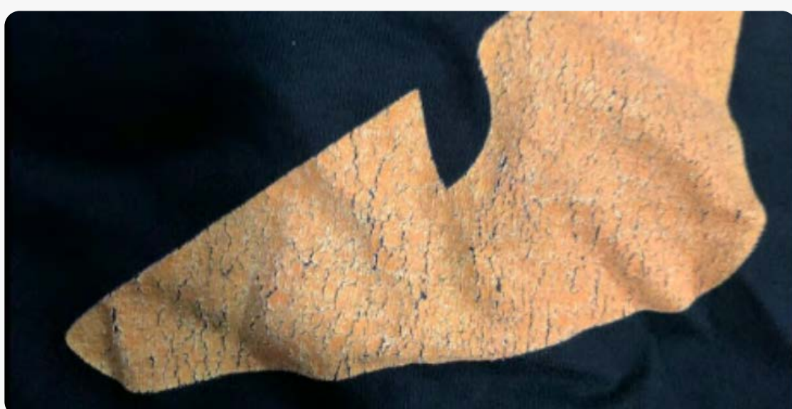
Cracks appearing after wash
